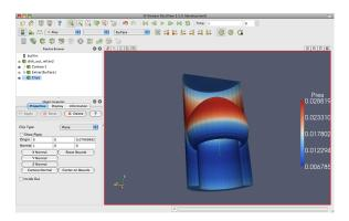
If you have a contour, you should now see the isosurface contour within a cutaway of the mesh surface. You will probably have to rotate the mesh to see the contour clearly.
