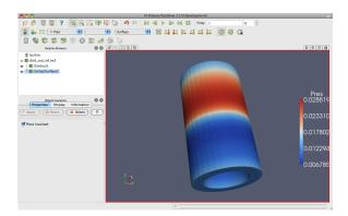
When you apply the Extract Surface filter, you will once again see the surface of the mesh. Although it looks like the original mesh, it is different in that this data is hollow whereas the original data was solid throughout.
