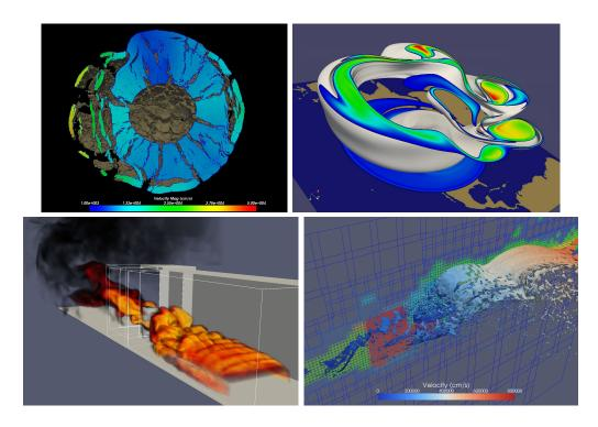
ParaView is used frequently at Sandia National Laboratories for visualizing data from large-scale simulations run on the Red Storm supercomputer such as the examples shown here. The upper left image shows a CTH shock physics simulation with over 1 billion cells of a 10 megaton explosion detonated at the center of the Golevka asteroid. The upper right image shows a SEAM Climate Modeling simulation with 1 billion cells mod-
