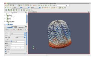
Now the streamlines are augmented with little pointers. The pointers face in the direction of the velocity, and their size is proportional to the magnitude of the velocity. Try using this new information to answer the following questions.
