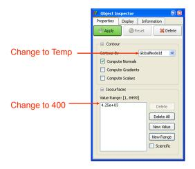
We will use the contour filter to create an isosurface where the temperature is equal to 400 K. First, change the Contour By parameter to the Temp variable. Then, change the isosurface value to 400. Finally, hit value will see the isosurface appear inside of the volume. If disk\_out\_ref.ex2 was still colored by pressure from Exercise 2.5, then the surface is colored by pressure to match.
