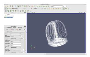
The surface of the mesh is replaced with some swirling lines. These lines represent the flow through the volume. Notice that there is a spinning motion around the center line of the cylinder. There is also a vertical motion in the center and near the edges.
