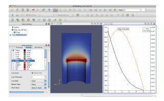
From this plot we can verify some of the observations we made in Section 2.5. We can see that the temperature is maximal at the plate surface and falls as we move away from the plate, but the pressure goes up and then back down. In addition, we can observe that the maximal pressure (and hence the location where the forces on the air are equalized) is 2.74 units away from the disk.
