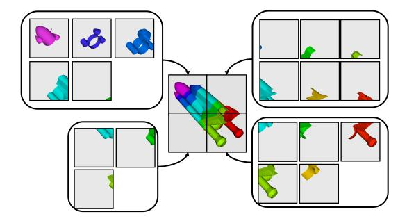
IceT also has the ability to drive tiled displays, large, high-resolution displays comprising an array of monitors or projectors. Using a sort-last algorithm on a tiled display is a bit counterintuitive because the number of pixels to composite is so large. However, IceT is designed to take advantage of spatial locality in the data on each process to drastically reduce the amount of compositing necessary. This spatial locality can be enforced by applying the D3 filter to your data.
