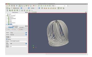
You can now see the streamlines much more clearly. As you look at the streamlines from the side, you should be able to see circular convection as air heats, rises, cools, and falls. If you rotate the streams to look down the Z axis at the bottom near where the heated plate should be, you will also see that the air is moving in a circular pattern due to the friction of the rotating disk.
