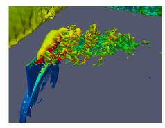
A PHASTA simulation of 3.3 billion tetrahedral cells involving the flow over a full wing where a synthetic jet issues an unsteady crossflow jet.
